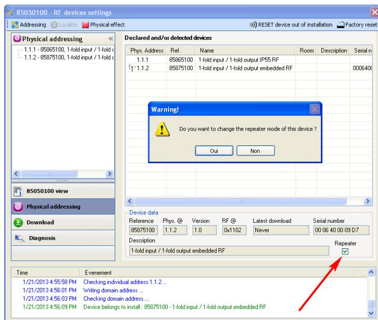
To activate the Repeater function, tick the repeater box on the physical addressing screen of the product concerned.
