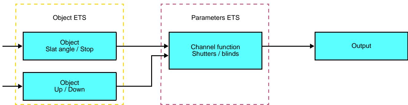
This function is used to control a shutter or blind using two push buttons (Inputs). One button for Up and one button for down. The function transmits the **Up / Down** object (long key press) and the **Slat angle adjustment / Stop** object (short key press).
