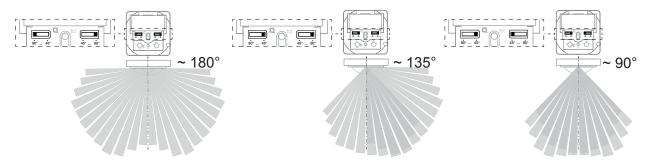
Fig. 8: Setting the detection angle
