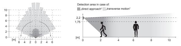
Figure 7: detection area of the motion detector for mounting height 2.2 m
