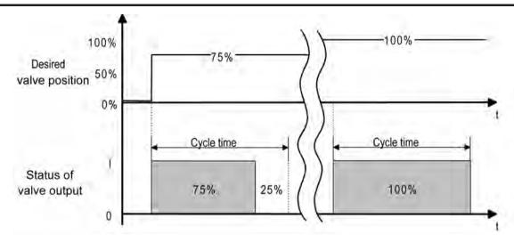
picture 11: Conversion of a constant valve setpoint position to an output signal with deenergised, closed valve drives (example)
