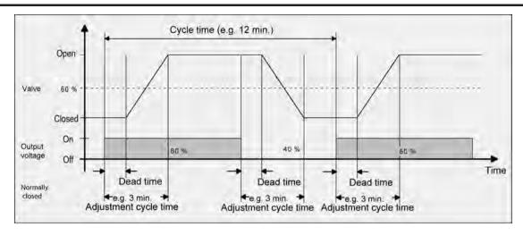
picture 23: Ideal course of the valve stroke for a command value of approx. 60 % of a deenergised, closed valve
