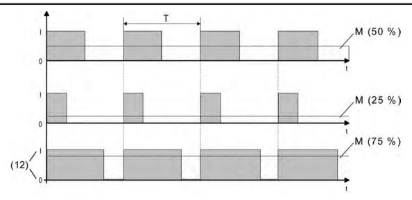
picture 16: Pulse width modulation of a valve output signal
