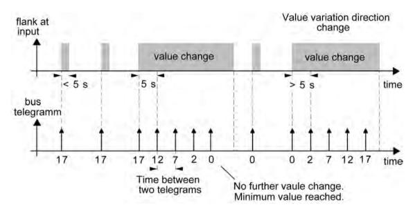
picture 8: Example to change the value for dimming value encoder
