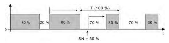
picture 18: Command value change, e.g. from 80 % to 30 % during the closing phase of the
