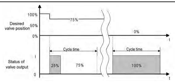
picture 13: Conversion of a constant valve setpoint position to an output signal with deenergised, opened valve drives (example)
