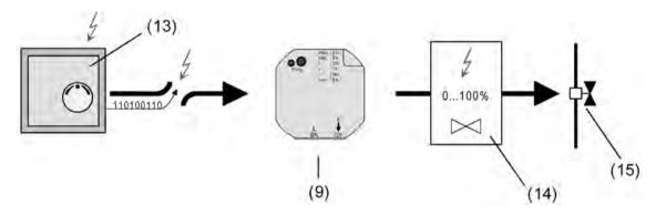
picture 25: Principle of cyclical command value monitoring in the event of a fault (e.g. open circuit)
