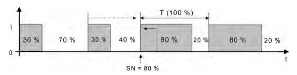
picture 22: Command value change, e.g. from 30 % to 80 % during the closing phase of the valve (closing phase too long)
