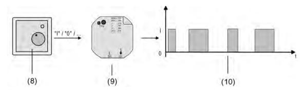
picture 14: Command value principle for switching command value
