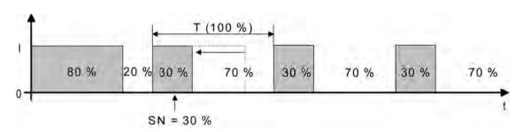
picture 17: Command value change, e.g. from 80 % to 30 % during the opening phase of the valve
