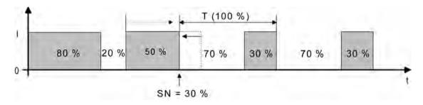
picture 19: Command value change, e.g. from 80 % to 30 % during the opening phase of the valve (opening phase too long)
