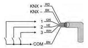
picture 5: Connection of the extension inputs
