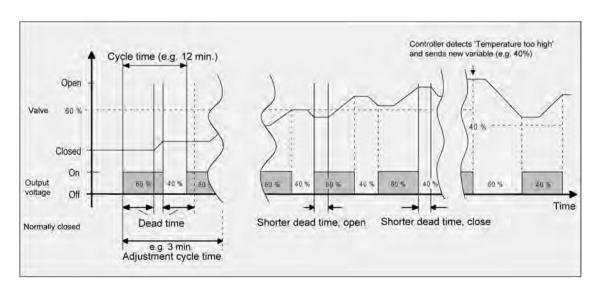
picture 24: Ideal course of the valve stroke for a command value of approx. 60 % at first of a deenergised, closed valve
