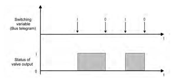
picture 10: Conversion of a switching command value to an output signal with deenergised, closed valve drives (example)
