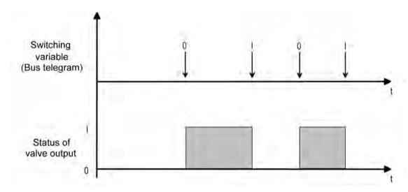
picture 12: Conversion of a switching command value to an output signal with deenergised, opened valve drives (example)
