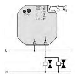
picture 4: Connection of the mains voltage and the load
