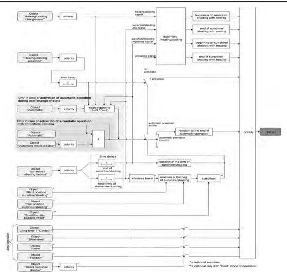
picture 49: Function diagram of automatic heating/cooling
