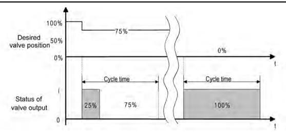
picture 54: Conversion of a constant valve nominal position into an output signal with valve drives that are open when deenergized (example)
