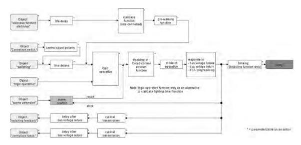
picture 22: Functional diagram of the scene function
