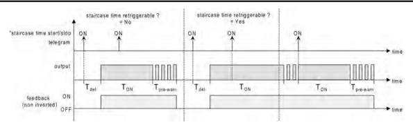
picture 18: Switch-on behaviour of the staircase function
