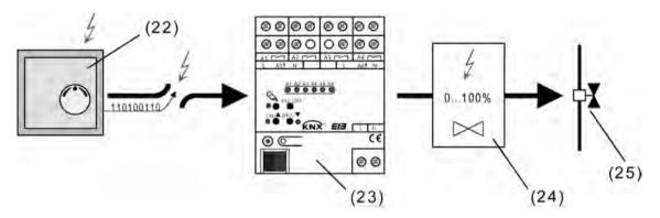
picture 67: Principle of cyclical command value monitoring in the event of a fault (e.g. open circuit)
