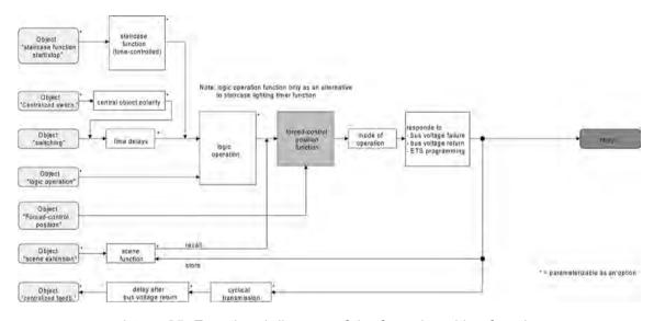
picture 25: Functional diagram of the forced position function
