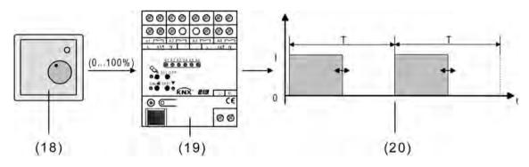
picture 57: Command value principle with constant command value
