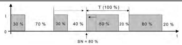
picture 64: Command value change e.g. from 30 % to 80 % during the closing phase of the valve (closing phase too long)
