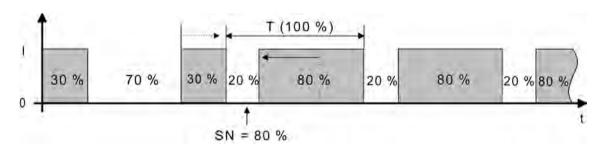
picture 63: Command value change e.g. from 30 % to 80 % during the closing phase of the valve
