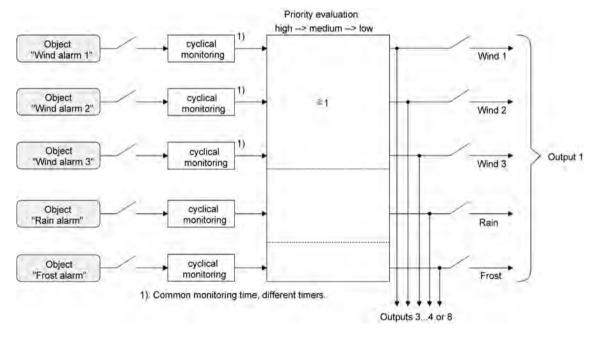
picture 13: Function diagram of the safety function
