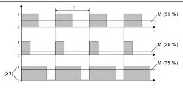
picture 58: Pulse-width modulation of a valve output signal
