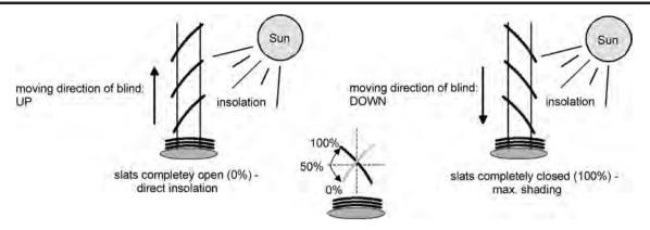
picture 30: type 1 - slatted blinds with oblique slat position in both travel directions
