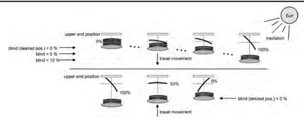
picture 34: Example of slat positioning with the blind in upper end position (typical of slat type 1.)
