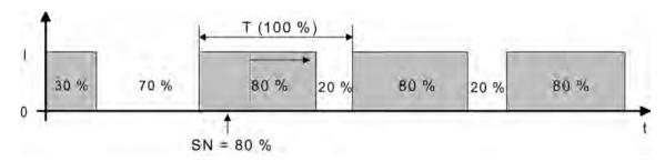
picture 62: Command value change e.g. from 30 % to 80 % during the opening phase of the valve
