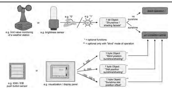
picture 38: Schematic diagram illustrating the simple sun protection configuration
