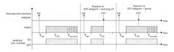
picture 19: Switch-off behaviour of the staircase function
