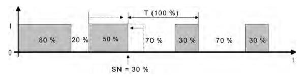
picture 61: Command value change e.g. from 80 % to 30 % during the opening phase of the valve (opening phase too long)
