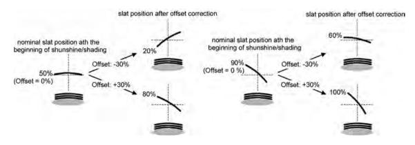
picture 42: Functional principle of slat offset (typical of slat type 1; analogous reaction for slat type 2)
