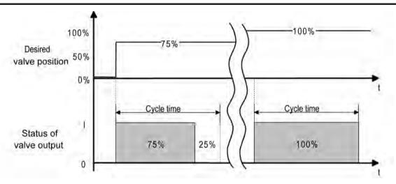
picture 52: Conversion of a constant valve nominal position into an output signal with valve drives that are closed when deenergized (example)
