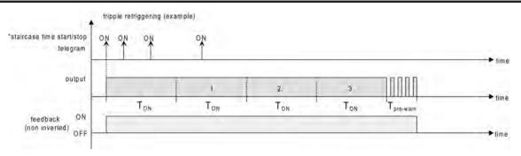
picture 21: Time extension for staircase function
