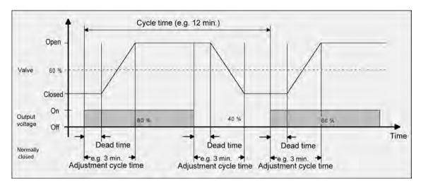
picture 65: Idealised curve of the valve stroke: example for a command value of approx. 60 % for a valve closed when deenergized
