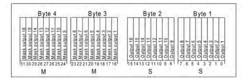
picture 11: Structure of the centralized feedback object
