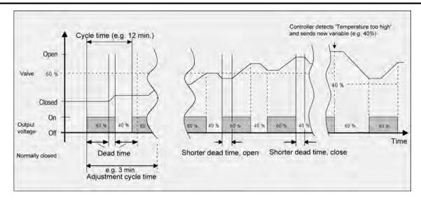
picture 66: Idealised curve of the valve stroke: example for an initial command value of approx. 60 % for a valve closed when deenergized
