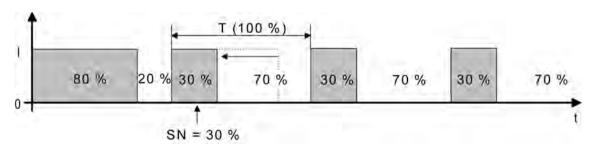
picture 59: Command value change e.g. from 80 % to 30 % during the opening phase of the valve
