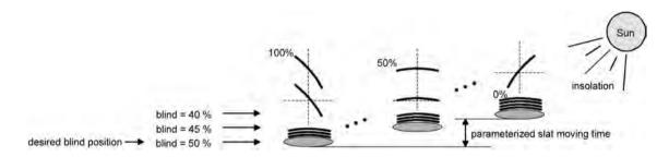
picture 33: Example of slat positioning affecting the position of the blind (typical of slat type 1; analogous reaction for type 2.)
