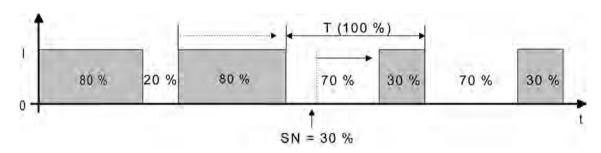
picture 60: Command value change e.g. from 80 % to 30 % during the closing phase of the valve
