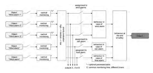
picture 36: Function diagram of channel-oriented safety functions
