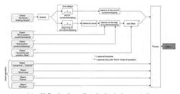
picture 39: Function diagram illustrating the simple sun protection
