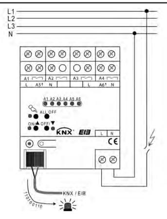
picture 8: Monitoring of the mains voltage
