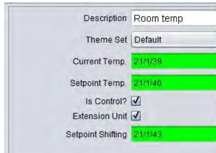
Fig. 91: Mobile Editor - Parameterisation window
