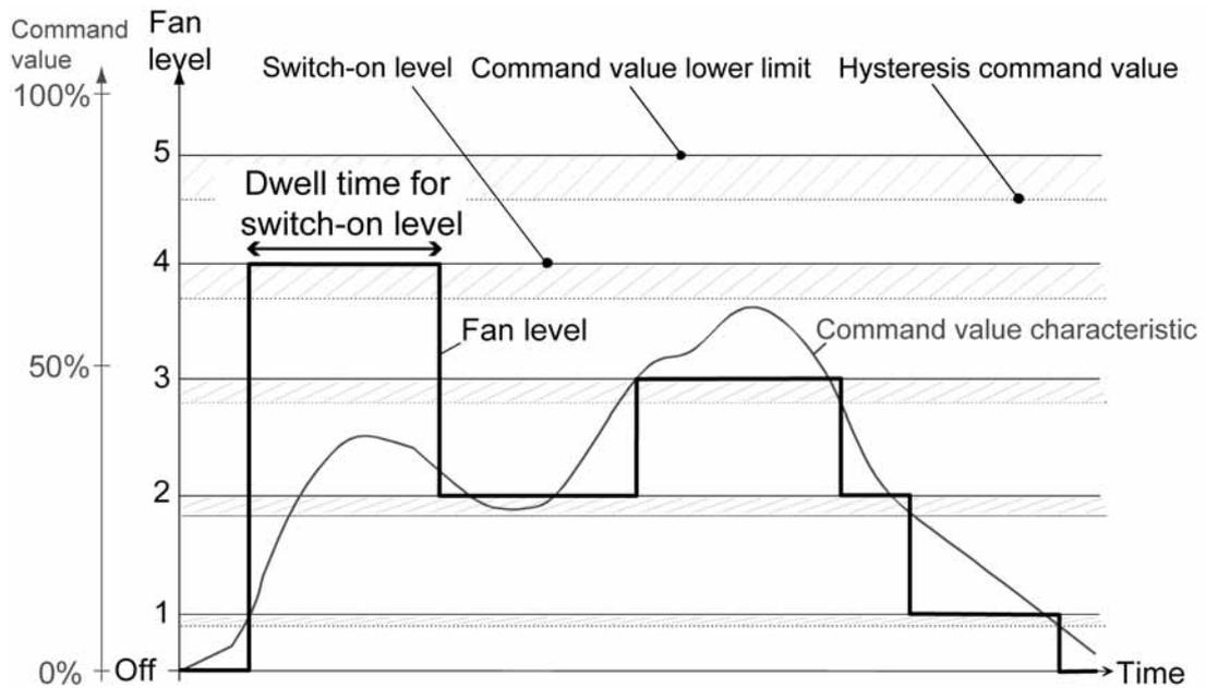
picture 22: Simplified command value diagram to illustrate a fan level change-over (active fan level), taking into account the switch-on level
