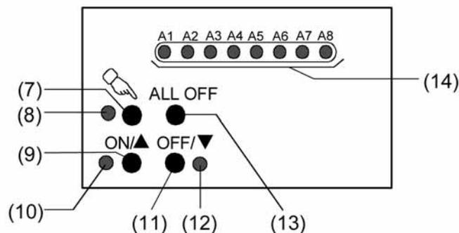
picture 6: Controls and indicators for manual control
