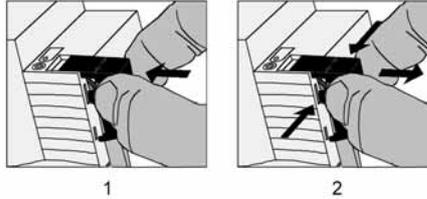
picture 5: Installing / removing the protective cap
