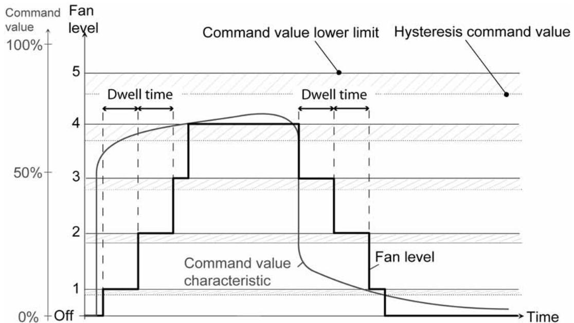
picture 26: Simplified command value diagram to illustrate a fan level change-over with the level principle, taking into account the dwell time
