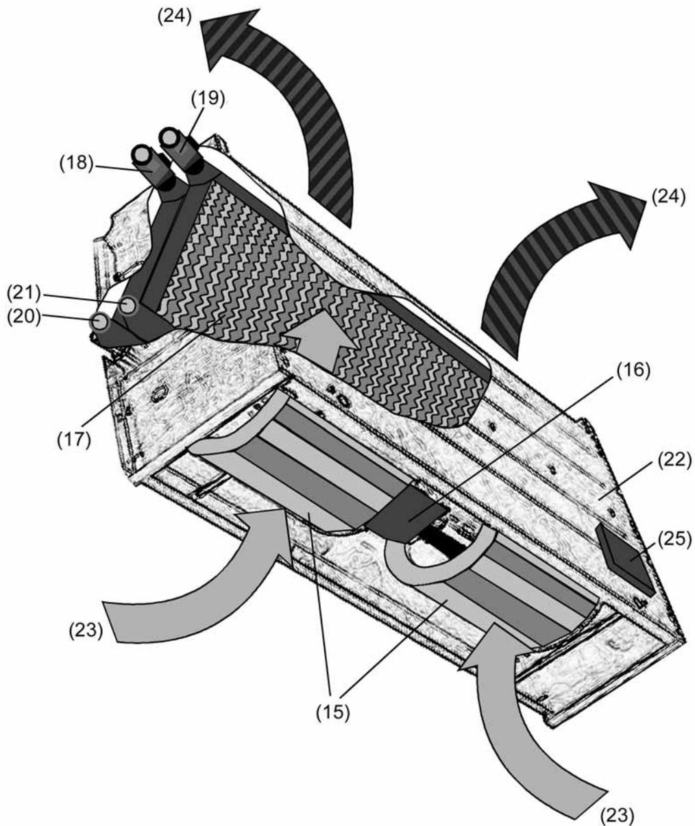
picture 7: The fan coil principle (example based on a 4-pipe fan coil unit with upright design)
