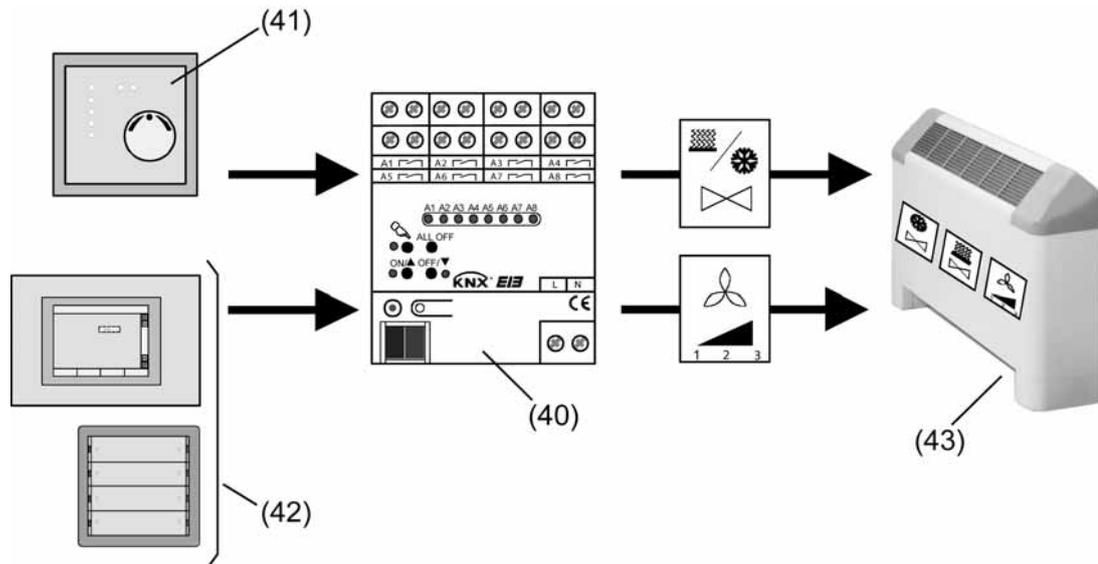
picture 28: Principle of manual fan control
