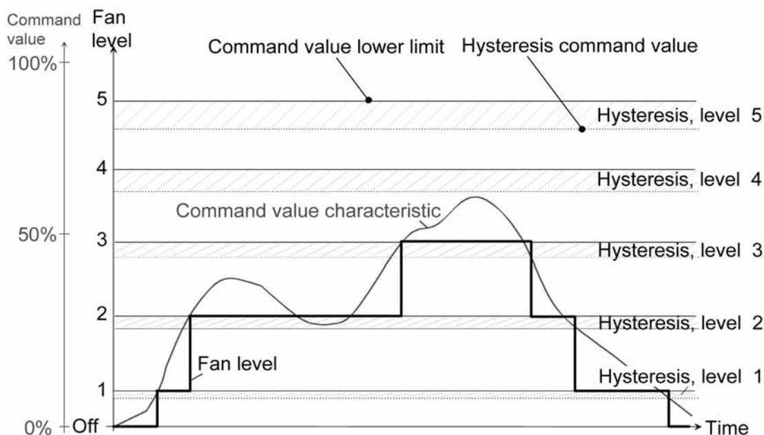
picture 21: Simplified command value diagram to illustrate a fan level change-over (active fan level), taking into account the command value lower limits and the hysteresis
