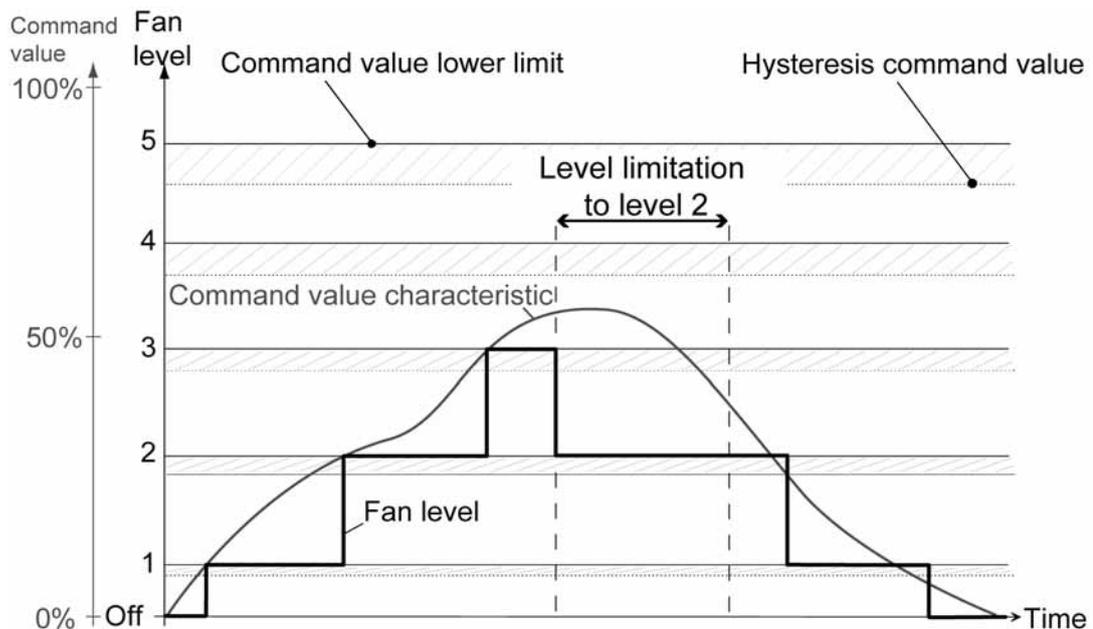
picture 27: Simplified command value diagram to illustrate the reaction to a fan level limitation
