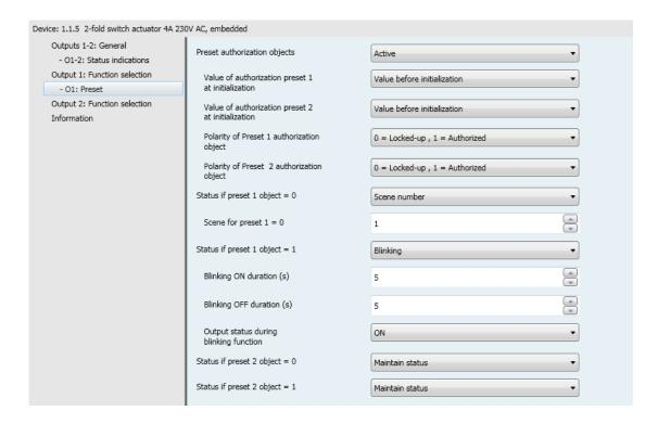
The Preset function is used to switch an output into various predefined states. The preset function is activated via 1-bit format objects.
