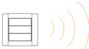
A Push-button 3gang with wall-mounted transmitter insert
