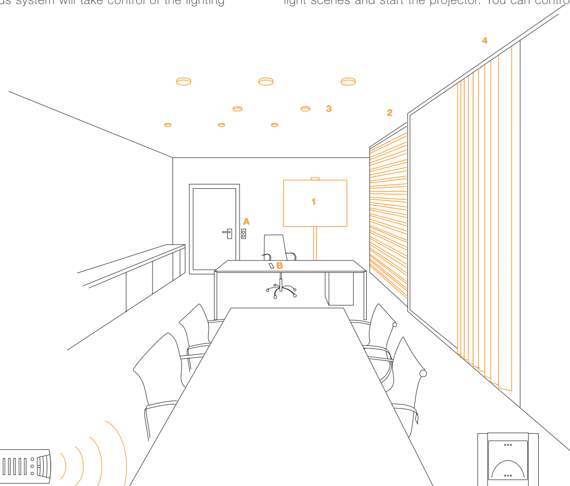
B Hand-held radio transmitter with 5 light scene buttons
