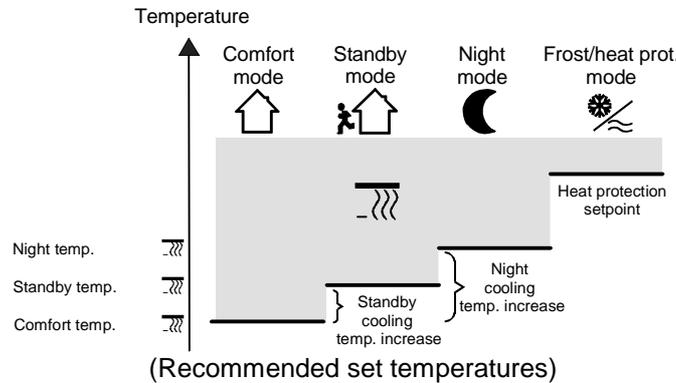
The set-temperatures for comfort, standby and night mode exists for this heating/cooling mode. The heat protection temperature can be preset. The following applies:
