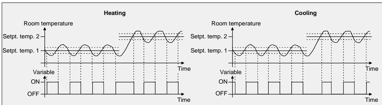
An additional 2-point control heating or cooling stage works exactly the same as the 2-point control of the basic stage. The difference is that the setpoint and the hystereses values will shift by taking into account the parameterized stage offset.
