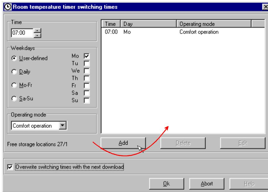
This way it is possible to pre-program up to 28 switching programmes. A programme created in the right part of the window may be edited by highlighting it and clicking the „Edit“ button. Highlighting the programme and clicking the „Delete“ button will delete the programme and remove it from the list. Clicking the „OK“ button will accept the settings into the projection of the push button.
