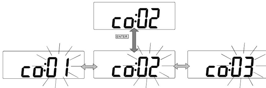
The contrast value can be adjusted in negative or positive direction (min. „co:00“ / max. „co:10“) by pressing the left or right display key.
