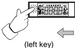
Selecting a menu item by navigating to the left or adjusting a value (e.g. temperature value or switching time) in negative direction. During 'normal operation' (no programming mode is activated) the setpoint can be shifted via this key (does not apply to the controller extension)
