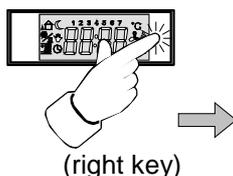
Selecting a menu item by navigating to the right or adjusting a value (e.g. temperature value or switching time) in positive direction. During 'normal operation' (no programming mode is activated) the setpoint can be shifted via this key (does not apply to the controller extension)
