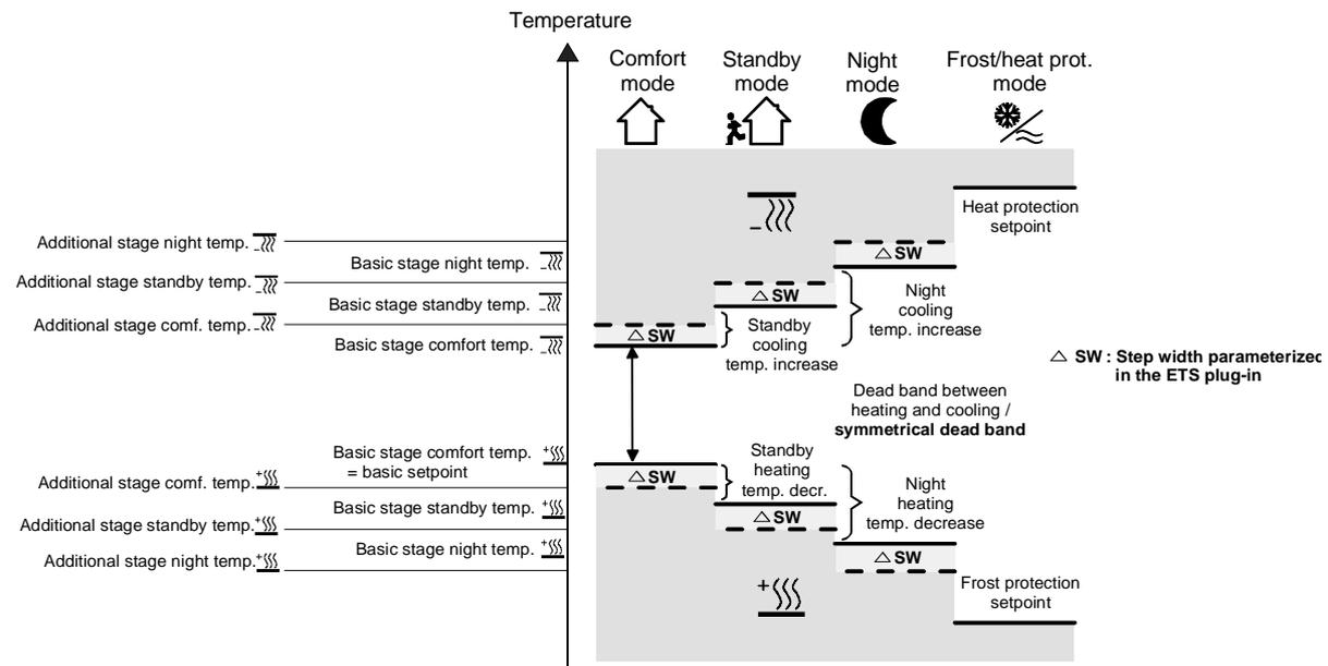
$$T_{\text{Comfort set value additional stage heating}} \leq T_{\text{Comfort set value basic stage heating}} \leq T_{\text{Comfort set value basic stage cooling}} \leq T_{\text{Comfort set value additional stage cooling}}$$
