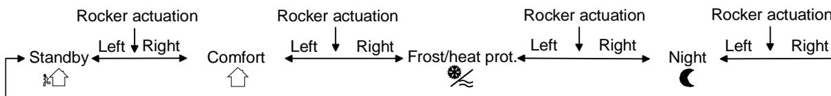
It is not possible to activate a comfort mode extension (presence function) with a rocker function!
