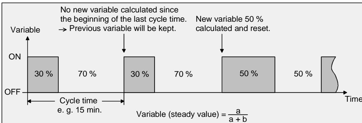
With an actuating variable of 0 % (continuously switched-off) or 100 % (continuously switched-on) an actuating variable telegram according to the actuating variable value ("0" or „1“) is output after a cycle time has elapsed. With this type of control the 'clipping' (cf. „continuous PI control“) is active as well.
