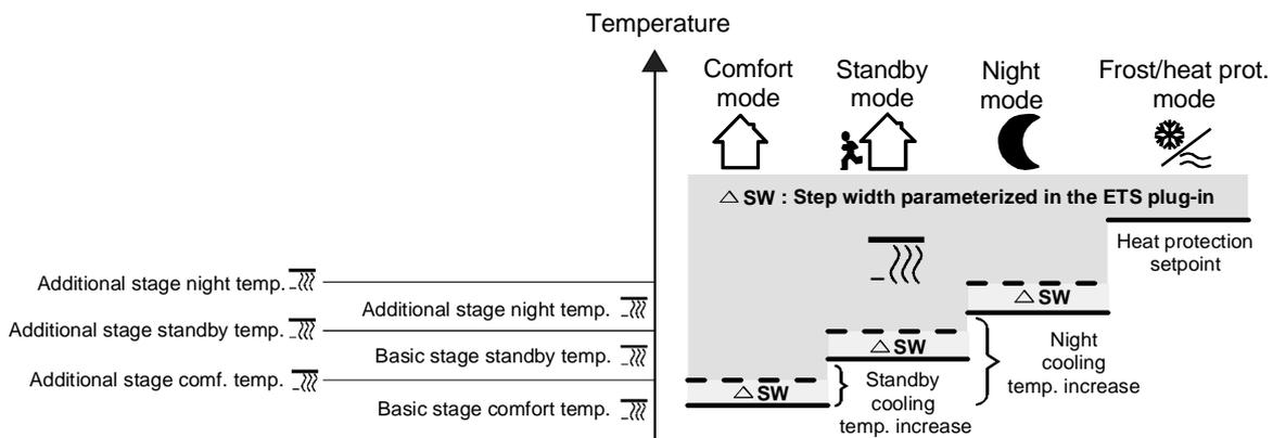
$$T_{\text{Comfort set value basic stage cooling}} \leq T_{\text{Comfort set value additional stage cooling}} / T_{\text{Standby set value basic stage cooling}} \leq T_{\text{Standby set value additional stage cooling}}$$
