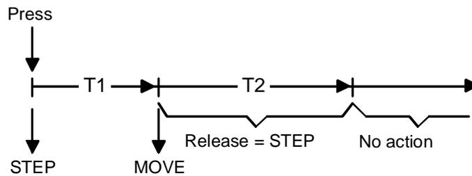
Pressing a rocker's key will transmit a step command and time T1 is started ("time between step and move operation") No other telegram is transmitted, if the key is released within T1. This step serves to stop a continuous run in progress.
