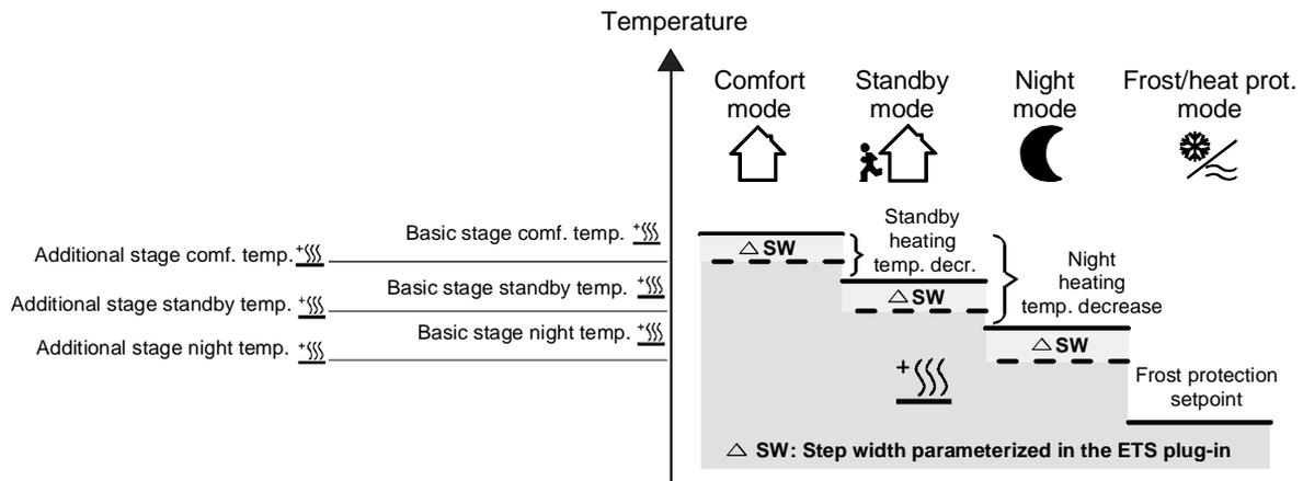
$$T_{\text{Comfort set value additional stage heating}} \leq T_{\text{Comfort set value basic stage heating}} / T_{\text{Standby set value additional stage heating}} \leq T_{\text{Standby set value basic stage heating}}$$
