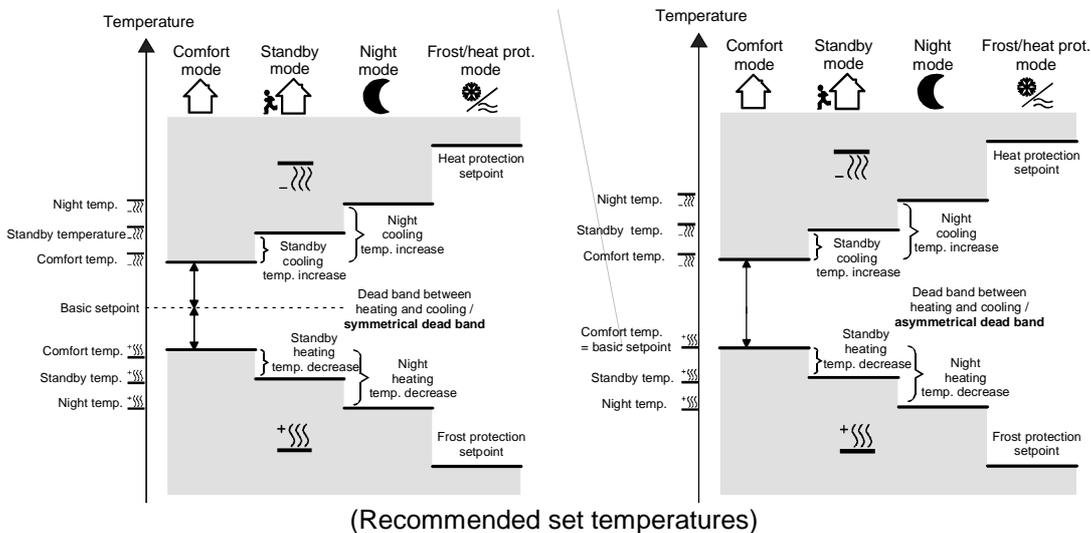
For this heating/cooling mode, the set-temperatures of both heating/cooling modes exist for comfort, standby and night mode as well as the Dead band. In addition, the frost protection and the heat protection temperatures can be preset. The following applies:
