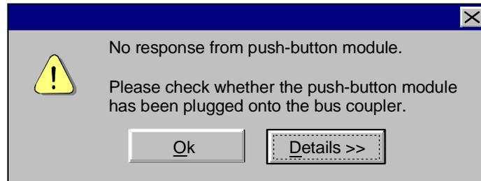
**Appears:** When trying to load the application data into the device.
