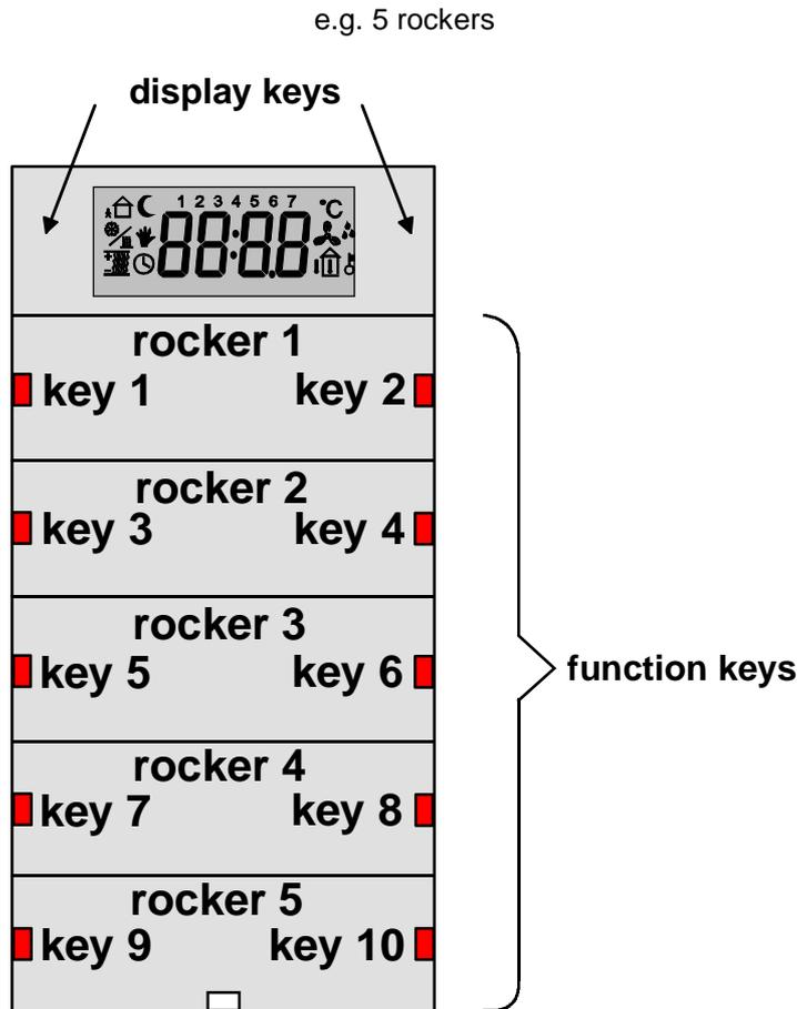
Depending on the application included in the ETS project (2 gang, 3 gang or 5 gang) the required number of rockers and LED's is automatically applied in the ETS plug-in.
