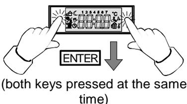
Accessing the programming menus (pressing the keys for at least 3 sec) or confirming a preset value such as setpoint or switching time (pressing the keys for at least 1 sec)
