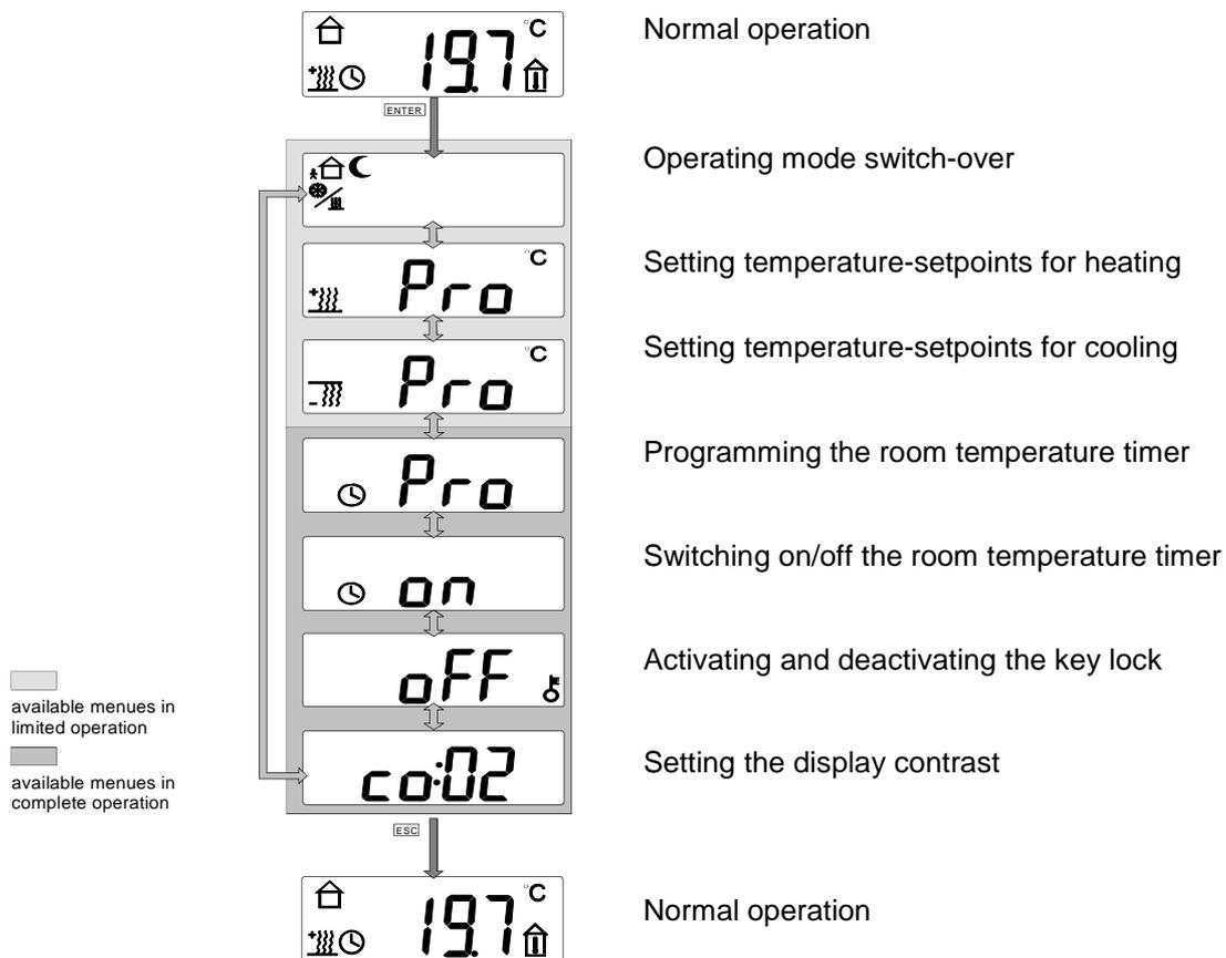
The programming mode is accessed by pressing both display keys for approx. 3 sec. This will activate the main menu. The display keys can be used here to navigate between the individual menu items. The corresponding submenus to the selected menu can be accessed by pressing both display keys ("Enter").
