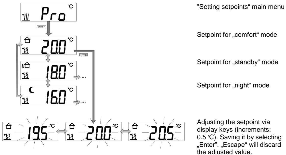
Once a setpoint has been set and the input has been confirmed by an Enter command, the operating mode associated with the adjusted setpoint will be accepted as the active mode. This, however, is only the case if no higher-priority mode (e.g. window contact / presence detector) is activated or if the KONNEX forced object is not activated!
