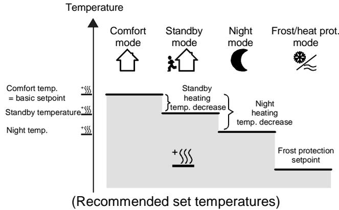
The set-temperatures for comfort, standby and night mode exists for this heating/cooling mode. The frost protection temperature can be preset. The following applies:
