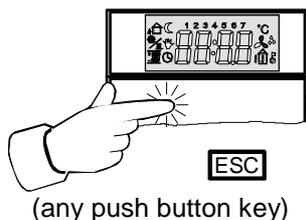
The programming mode or the selected menu (return into the higher-level menu) may be left by pressing any push button key (not the display keys). The escape command will discard any readjusted value. In this case the readjusted value will not be accepted in the memory of the device.
