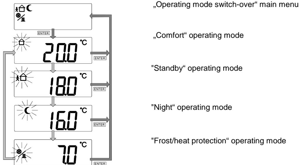
The operating mode selected via the display keys will be accepted by the „Enter“ command. The display will subsequently switch back into the main menu.
