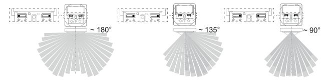
Fig. 8: Setting the detection angle
