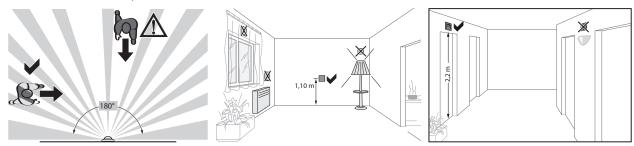
Fig 4: Installation location of the motion detectors
