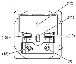
Fig. 5: Operating and adjustment elements of the bottom part of the application module
