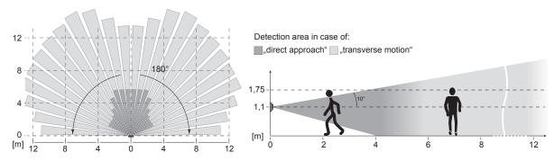
Figure 6: Detection area of the motion detector for mounting height 1.1 m
