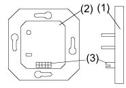
Attach the RTR touch sensor to the bus coupler using the locking screw (and also the additional screw for the 3-key and 5-key touch sensors).
