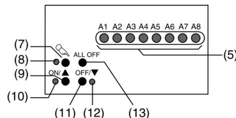
Fig. 2: Controls - layout
