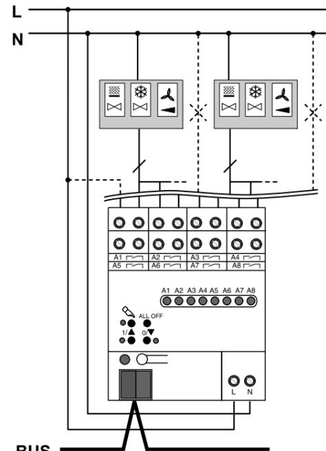
Fig. 6: connection of the load for 2 fan coil outputs
